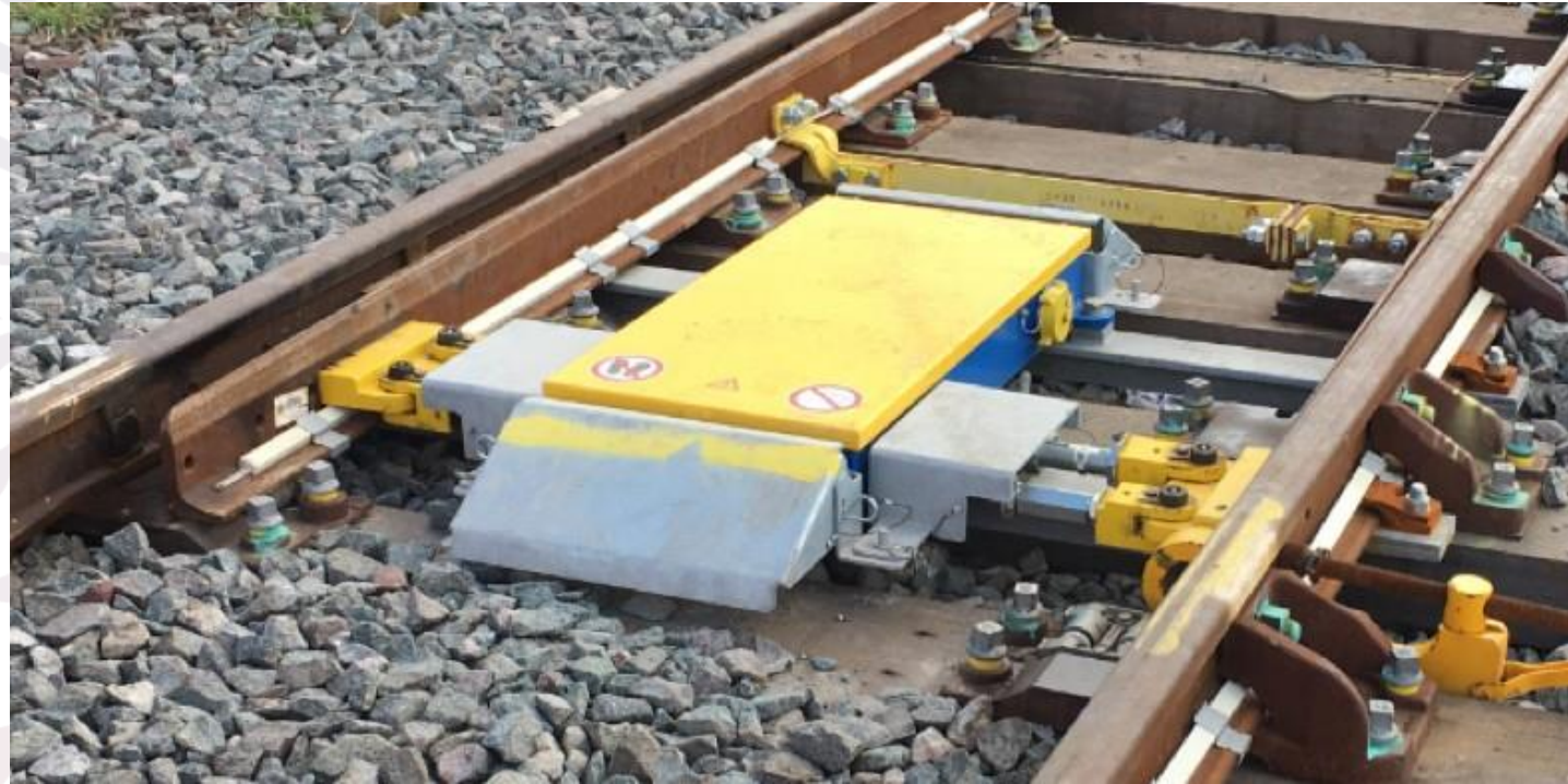
Figure 8 - Point machine installation
