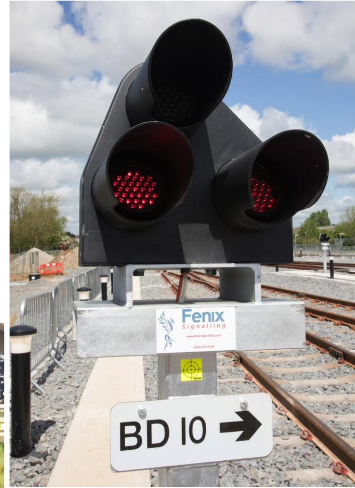
Figure 11 - Post mounted LED position light shunt signal
