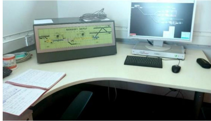
Figure 10 - VDU at Banbury Depot, UK (NR slot panel to left)
